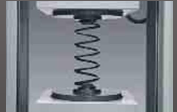
Spring test system with load measurement platform
