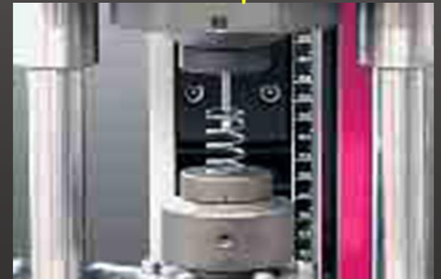
Precision Spring testing fixture for forces up to 500 N
