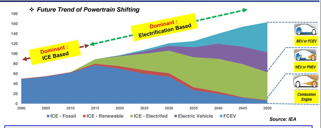
As an impact of stringent regulation of Fuel Economy / CO2, Global powertrain is predicted will shift from ICE Based to Electrification Based in the future.
